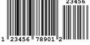
1 23456 78901 2 23456  | UPC-A allows for a supplemental two- or five-digit number to be appended to the main bar code symbol.                                                                                                                                                            |
