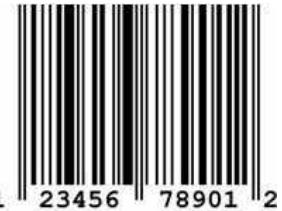
1 23456 78901 2         | UPC-A is a 12-digit numeric symbology consisting of 11 data digits and 1 check digit. The first digit is a number system that usually represents the type of product being identified.                                                                           |
