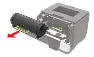
Remove the used imaging unit.
