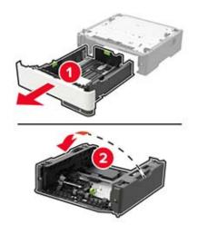
**5** Remove the used pick roller assembly.
