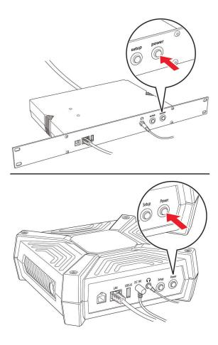
**Note:** The power button light starts blinking, and the indicator lights in the Ethernet port blink, go off, and then come on again.
