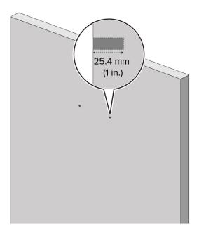
**5** Install 1.5-inch-long #6 standard wood screws into the holes, leaving about half an inch of the screws protruding. For Optra Compute CX2000, use #4 standard wood screws.
