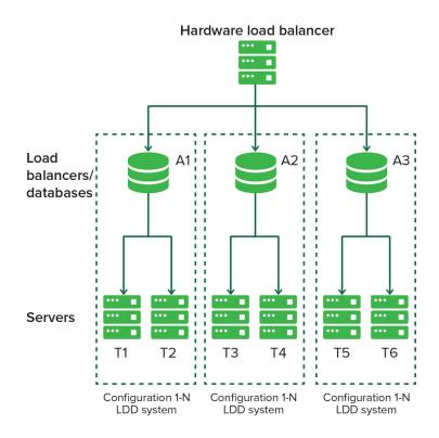
Each system group contains two identical LDD systems. Jobs are balanced between these systems in each group by the hardware load balancer or GSS. If one system fails, then the hardware load balancer or GSS directs jobs to other systems in the group until the failed system is online again.
