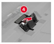
Remove the ADF separator roller.
