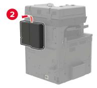
**5** Remove the controller board access cover.
