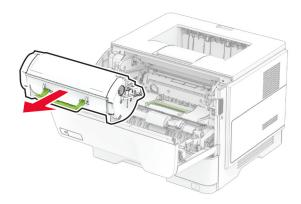
**3** Remove the used imaging unit.
