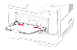
**5** From the control panel, set the paper size and paper type to match the paper loaded.
