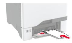
**Warning—Potential Damage:** Do not use envelopes with stamps, clasps, snaps, windows, coated linings, or self-stick adhesives.
