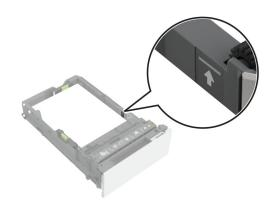
For envelopes and other specialty media, make sure that the stack height is below the dashed line. Overfilling may cause paper jams.
