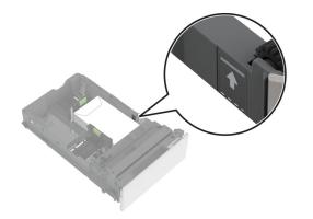
5 Insert the tray.If necessary, set the paper size and type to match the paper loaded in the tray.
