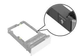
• For envelopes and other specialty media, make sure that the stack height is below the dashed line. Overfilling may cause paper jams.
