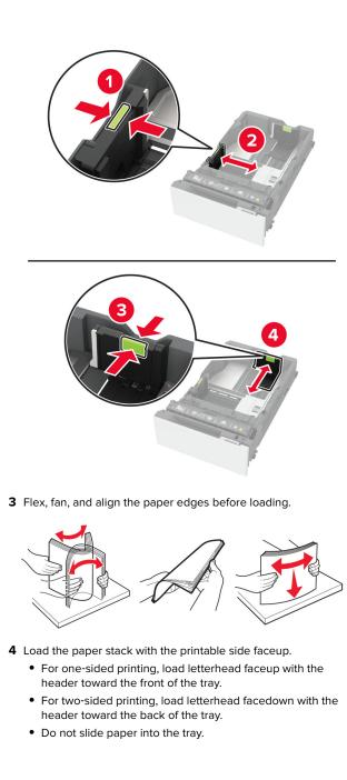
• For plain paper, make sure that the stack height is below the maximum paper fill indicator. Overfilling may cause paper jams.
