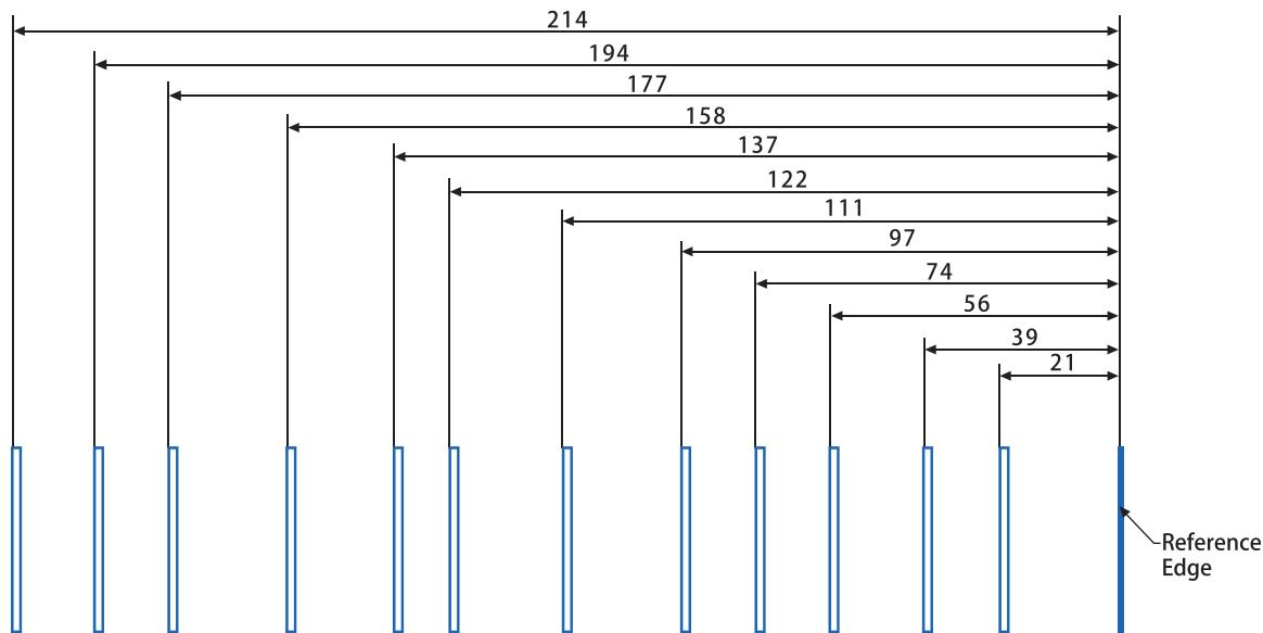
**Padrão de nervura para Lexmark B2865, M5255, M5265, M5270, MB2770, MS725, MS821, MS822, MS823, MS824, MS825, MS826, MX721, MX722, MX725, MX822, MX824, MX826, XM5365, XM5370, XM7355, XM7365, XM7370**
