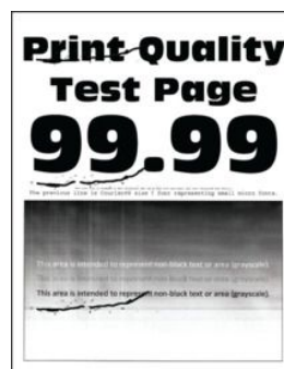
Repeating defects on page 407
