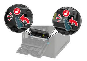
**3** Remove the used fuser.
