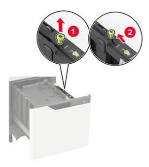
**b** If the A5 length guide is still attached, then remove it. If the guide is not attached, then proceed to <u>step</u> <u>d on page 31</u>.
