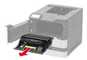
**4** Remove the used transfer roller.
