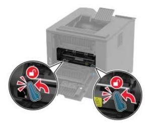
4 Remove the used hot roll fuser.
