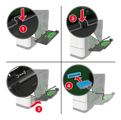
If a printer hard disk is installed, then remove the hard disk before installing the ISP.
