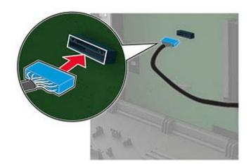
**6** Attach the hard disk to the controller board.
