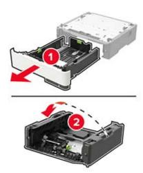
Remove the used pick roller assembly.
