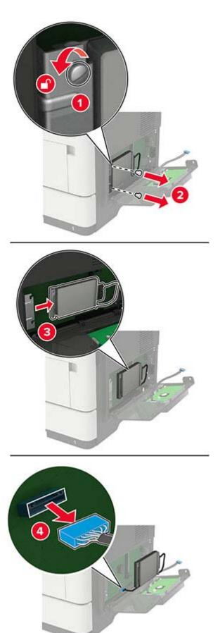
**b** Connect the ISP extended cable to the ISP connector.
