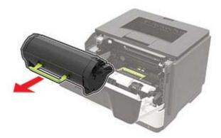
**3** Remove the used imaging unit.
