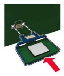
**Note:** The entire length of the connector on the card must touch and be flush against the controller board.
