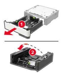
Remove the used pick roller assembly.
