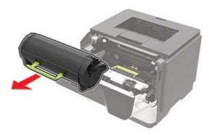
**3** Remove the used imaging unit.
