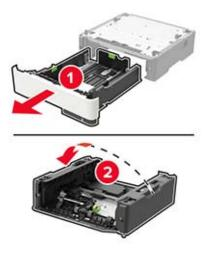
**5** Remove the used pick roller assembly.
