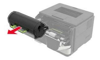
**3** Remove the used imaging unit.
