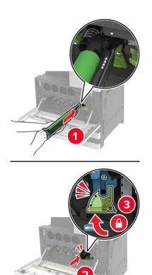
**6** Using the printhead wiper, clean the printhead lens.
