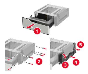
**12** Attach the side mounting brackets to the tray, and then insert the guide plate into the rail.
