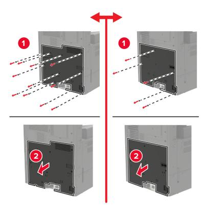
Remove the controller board shield.
