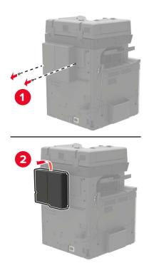
**11** Connect the finisher cable to the printer.
