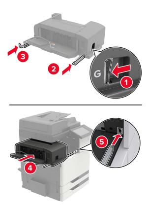
**10** Secure the finisher to the printer.
