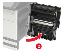
**3** Using the screwdriver stored inside door A, remove the door stopper.
