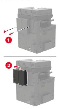
**5** Remove the controller board access cover.
