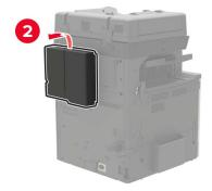
**5** Remove the controller board access cover.
