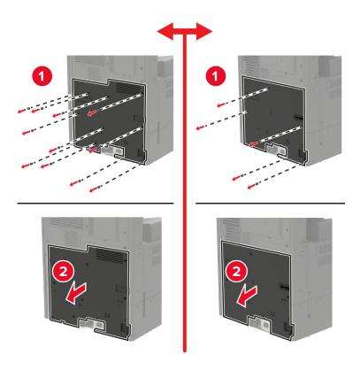
Remove the controller board shield.
