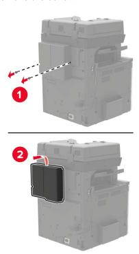
**5** Remove the controller board access cover.
