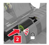
7 Insert the ADF separator roller cover until it *clicks* into place.
