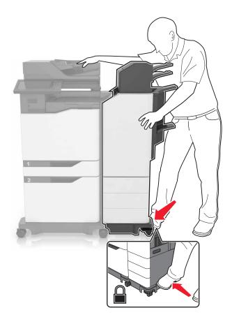
Check if the finisher and printer are properly locked by pulling hard the finisher away from the printer. If the finisher detaches from the printer, then repeat step 13 through step 14 until they are properly locked.
