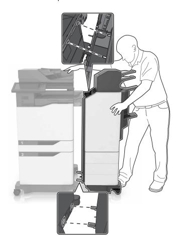
**14** Push the finisher to the printer by applying pressure at the bottom of the finisher until it *clicks* into place.
