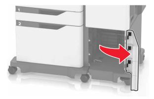
**b** Turn the levers of the finisher counterclockwise until the levers are loose.
