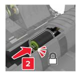
7 Insert the ADF separator roller cover until it *clicks* into place.
