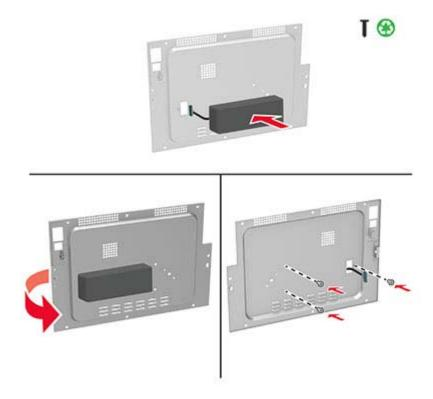
Connect the hard disk interface cable to the controller board, and then attach the access cover.
